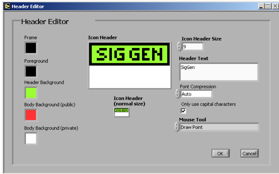
Figure 5. The front panel of Header Editor where header text and colors might be changed.
