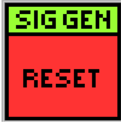
Figure 1. An example of an icon with a header. This icon has a green header background, red body background, black foreground (text color) and black frame color. All these colors are common for all VIs.
