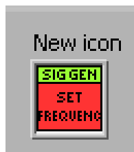
Figure 7. An example of an icon generation that was not perfect. This is common for VIs with long names (and words) where the text will not fit within the body.
